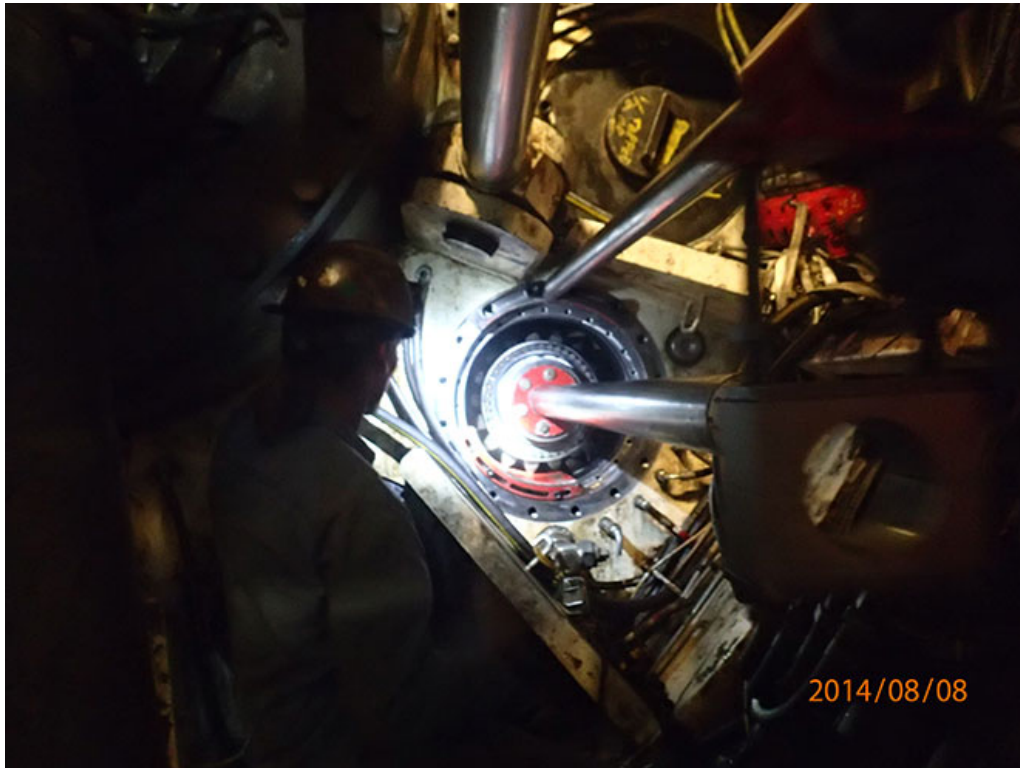
Performing repairs on the drive motor pinions
